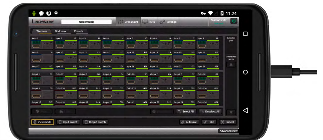
Tile View of the Crosspoint Menu of the Built-in Webpage (Displayed in a mobile device)
