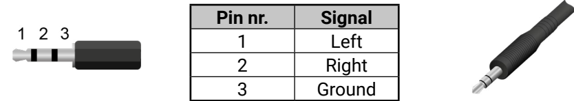
Jack audio plug pin assignments
