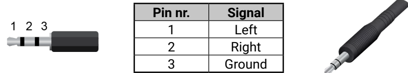
Jack audio plug pin assignments
